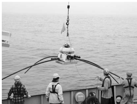
Figure 4. Deployment of a marine EM sensor (courtesy of AOA Geophysics, Inc.).
