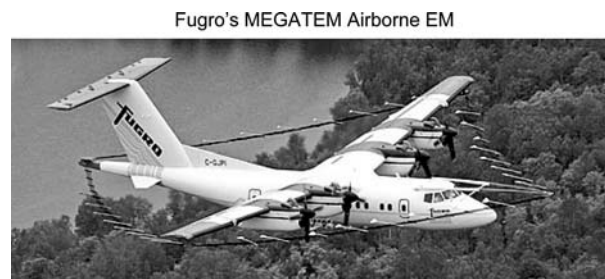
Figure 3. Fugro's MEGATEM AEM System.
